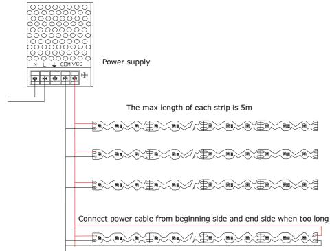
Note 8: When 5 meters strip is connected, please connect input cable from beginning side and end side at the same time to reduce brightness drop.
